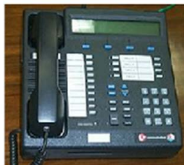
a) ISDN line; b) STE desk set. Note slot in front for Crypto PC Card and MLPP buttons
